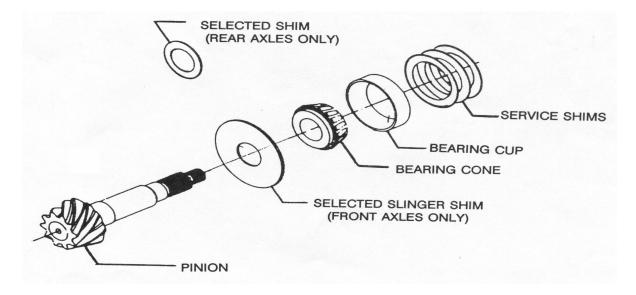
Axle assemblies are manufactured with a selective adjustment shim/slinger between the inner pinion bearing cone and pinion gear head. However, they may be serviced using the selective shim/slinger and/or shims placed in the carrier bore behind the inner pinion bearing cup. Refer to your vehicle service manual for proper procedures in determining the amount of shims required.
